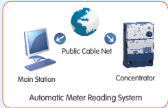
Automatic Meter Reading System
